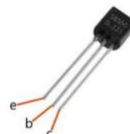
From these three regions, three poles are generated respectively, which are base (b), emitter (e), and collector (c). They form two P-N junctions, namely, the emitter junction and collection junction. The arrow in the circuit symbol indicates the direction of emitter junction. Transistors can be divided into two kinds: the NPN and PNP one. The former is made of two N-type semiconductors and one P-type and that
