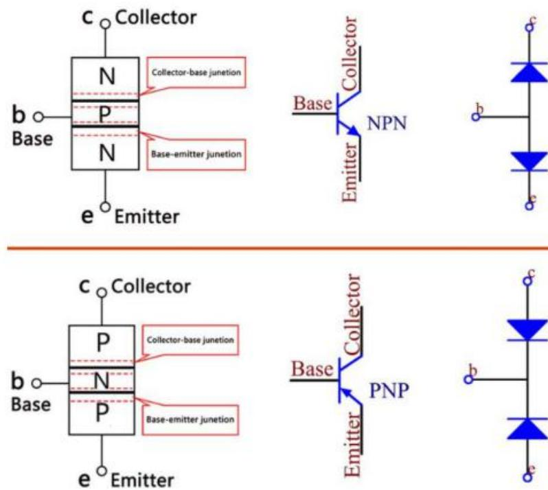
When a High level signal goes through an NPN transistor, it is energized. But a PNP one needs a Low level signal to manage it. Both types of transistor are frequently used for contactless switches, just like in this experiment.
